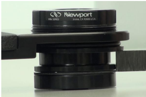
Figure 11 Gap tool thickness measurement showing correct preload.
