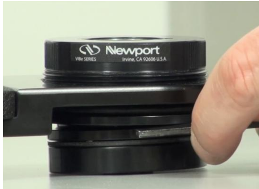
Figure 10 Gap tool thickness measurement showing overloaded condition
