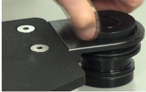
Figure 7 IB isolator height adjustment
