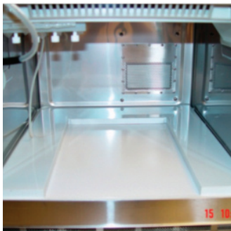
Sturdy, heat & chemical resistant guide allows exact placement of processing chamber every time.
