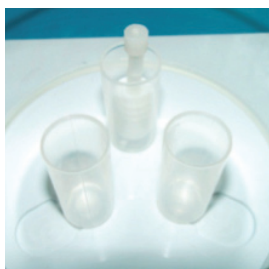
Lynx I specimen vial are locked in and tip-proof during processing. That's the specimen basket it holder assembly in the rear vial.
