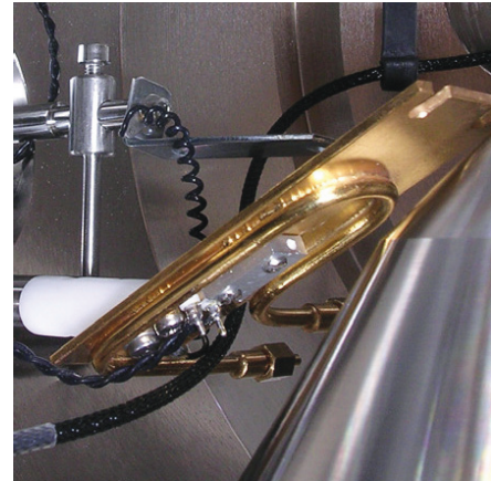
Cold trap - adapted to installation
