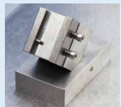
Pre-Frozen Sample Loading Jig
