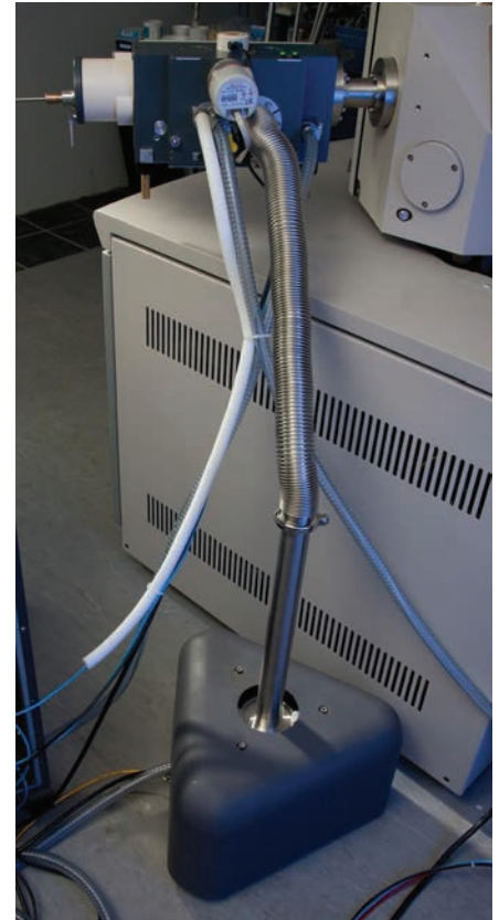
Remotely mounted turbomolecular pumping system
