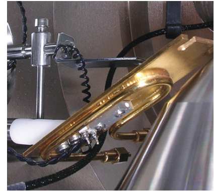
Cold trap - adapted to installation
