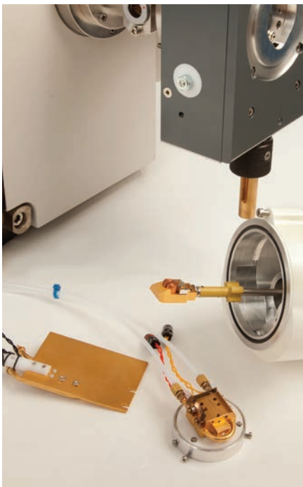
On-microscope components: airlock, cold stage, cold trap plus cryo transfer device
