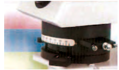
Analyzer with Bertrand Lens and Optical Compensators: full wave and ¼ wave
