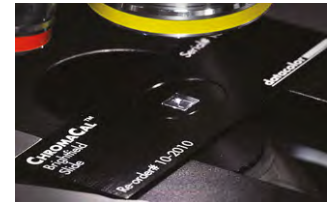
Color calibration slide on microscope stage
