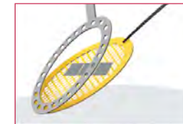
8. Separate the grid from the LOOP with an eyelash.
