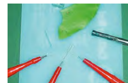
1.25 Uni-Core placing sample in pyrolysis gas chromatography tube
