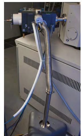
Remotely mounted turbomolecular pumping system
