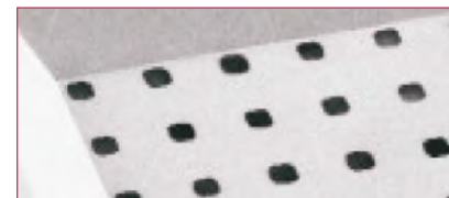
SEM image of a DuraSiN™ Mesh (taken from the back side)
