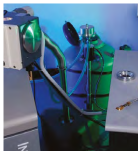
CHE3010 heat exchanger and dewar. During operation the heat exchange is inserted into the dewar. Typically hold times are up to 24 hours
