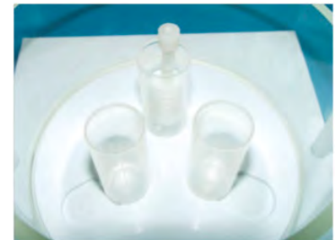
Lynx I specimen vial are locked in and tip-proof during processing. That's the specimen basket it holder assembly in the rear vial.
