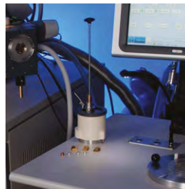
When not in use, the cryo transfer device can be stored under vacuum in the pumped storage tube, located on the Prepdek® work surface
