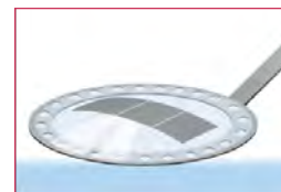
3. Gently lift up the LOOP with the sections in a droplet of water
