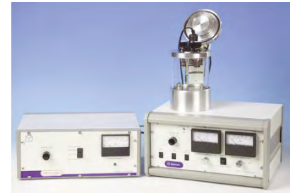
Optional carbon fibre evaporation attachment and controller
