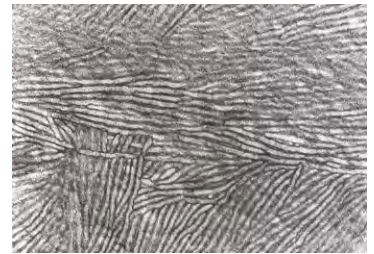
E. Ingolic, Technical University of Graz. Polymethylpenten, cryosection, RuO4 stained. X129000
