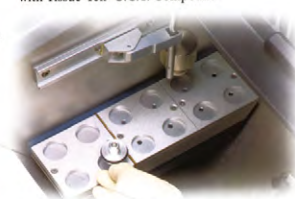
Place specimen on Cryobar®
