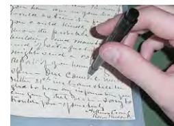
Using 2.0mm Uni-core to punch out ink sample
