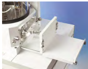
EMS 975 specimen drawer with stage in specimen exchange position
