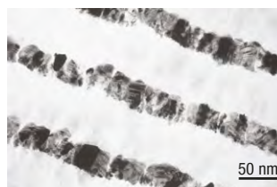
P. Swab, Advanced Refractory Technologies Inc., Buffalo, NY. ZnS/SiO 2 multilayer optical coating.
