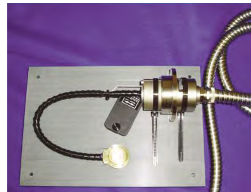
Coolstage and vacuum feed through connected to the storage block (with protection shutter open)
