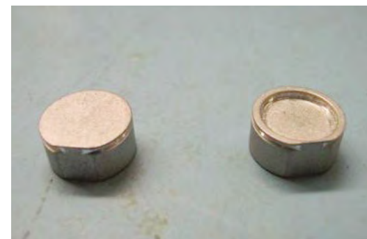
Dish-style specimen stub, showing flat bottom side (left) and dish side (right)
