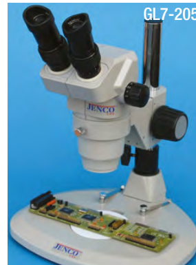
GL7-205 Post Stand has a slim, 1.25" / 35 mm, streamlined base for easy manipulation of large specimens Measures: 12" (w) (30cm) x 12" (h) (30cm) x 11" (d) (27cm)
