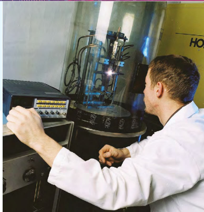
Hexaboride crystals are grown and purified in an inert gas atmosphere to specified crystal orientations.
