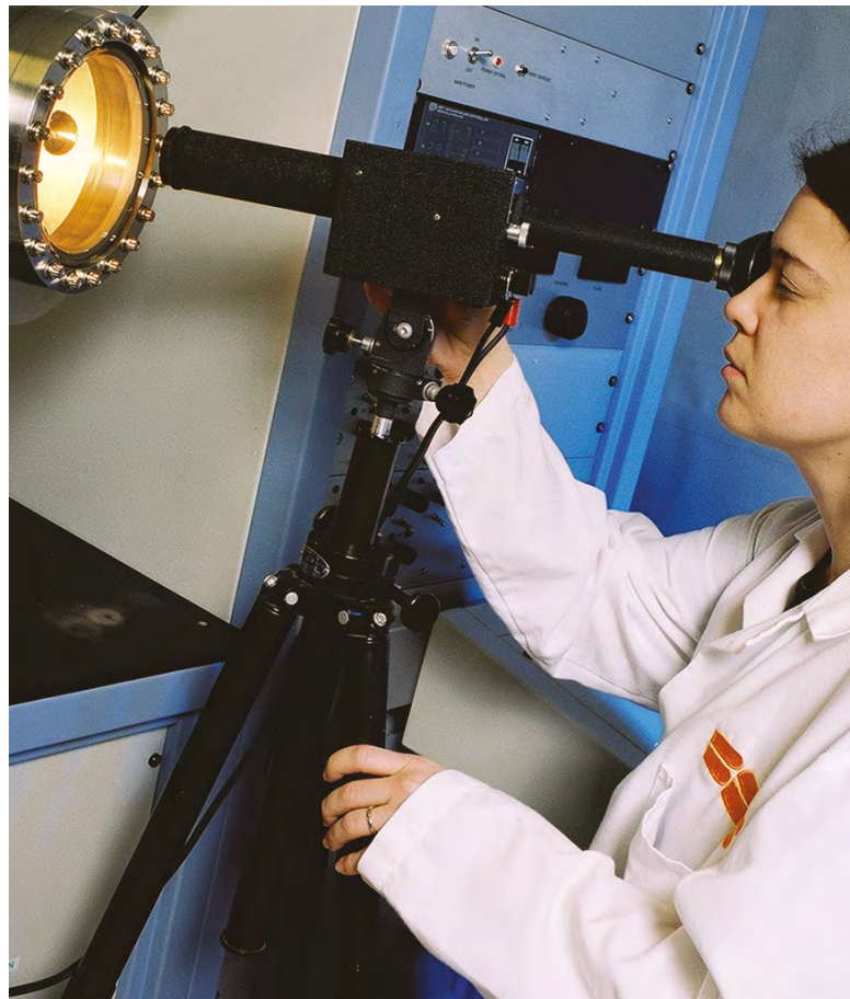
Hexaboride crystals are grown and purified in an inert gas atmosphere to specified crystal orientations.
