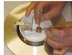
Transfer device, shuttle and universal specimen stub
