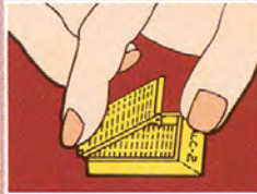
2. Press on back tab to open cover.
