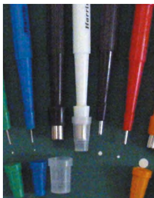
Using 2.0mm Uni-core to punch out ink sample
