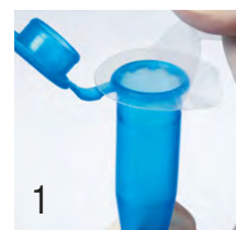
1 Remove the paper liner and adhere the membrane to the tube opening.
