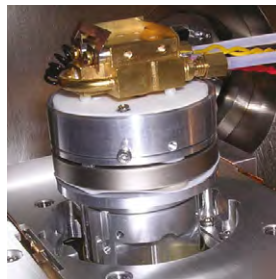
Nitrogen gas cooled cold stage—temperature range down to -190°C
