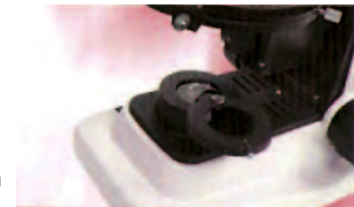
Polarizer slides in and out of light path above light collector
