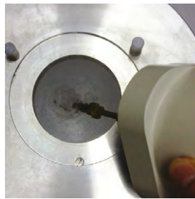
Plunge freezing in slushy nitrogen.
