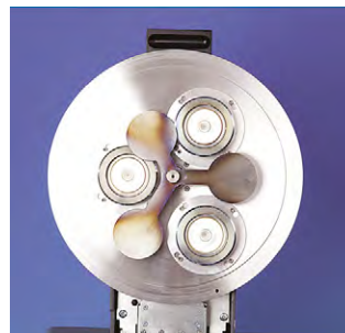
Triple sputtering head with automatic shutter open
