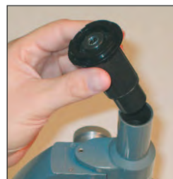
Simply thread the C-mount adapter on to the lens tube.
