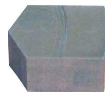
Micro- contour-artefact, calibrated by PTB
