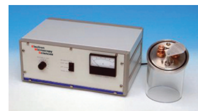
Optional carbon fibre evaporation attachment and controller (fitted)
