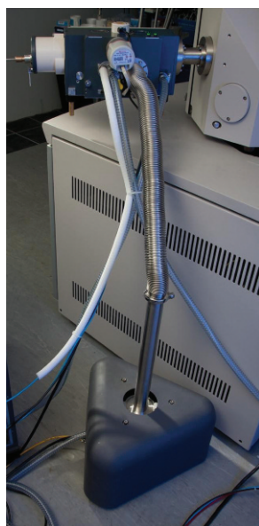
Remotely mounted turbomolecular pumping system
