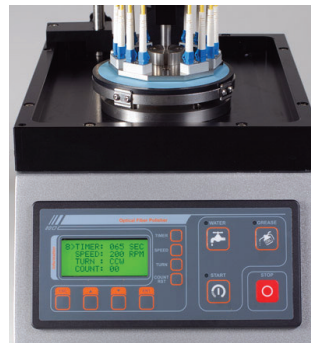
System has a handy station for resting connector holder during film changes.
