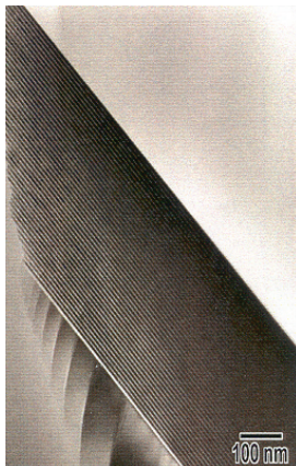
An X-ray mirror consisting of 45 layers of alternating Mo/Amorphous Si (7.0 nm period) on Si substrate. Image courtesy of John McCaffrey – National Research Council of Canada
