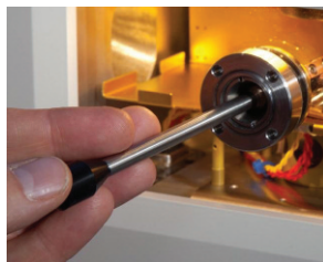
Front-mounted fracturing and specimen manipulation tool
