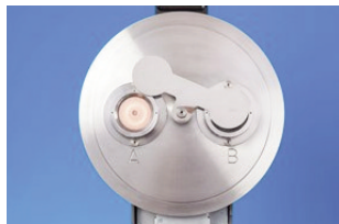
Dual sputtering heads and automatic shutter
