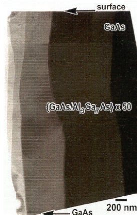
Multiple Quantum Well structure grown by MBE showing the thickness terraces possible with a MicroCleave™ sample. Courtesy of Scott Walk – Materials Directorate WPAFB. (Now with PPG Industries)
