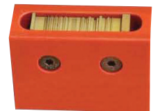
PTB calibrated micro artifact with steep flanks, height steps and cylindrical elements.
