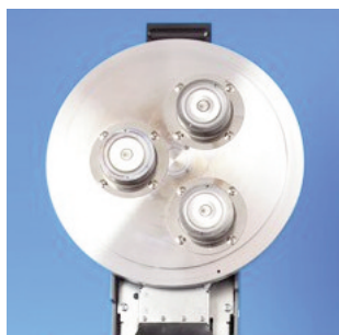
Triple sputtering head with automatic shutter open
