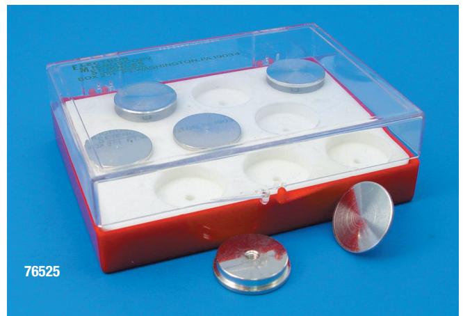
5) Sample Mount Storage Box A soft silicone base in a hinged plastic box; the base has 9 cavities, each 1" (25mm) in diameter and 1/4" (6mm) deep. Accommodates up to 9 mounting stubs of either 1" (25mm) in diameter or a 1/8" diameter pin.
