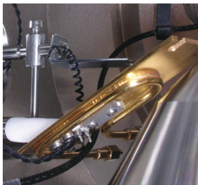
Cold trap - adapted to installation
