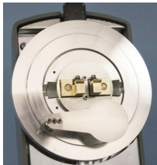
Carbon fiber evaporation insert and automatic source shutter
