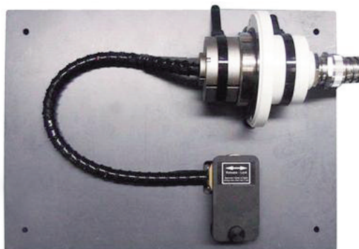
Coolstage and vacuum feed through connected to the storage block (stage protected by plastic shutter)
