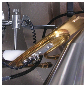
Cold trap - adapted to installation
