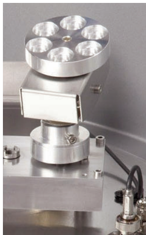
rotary planetary specimen stage (option)
