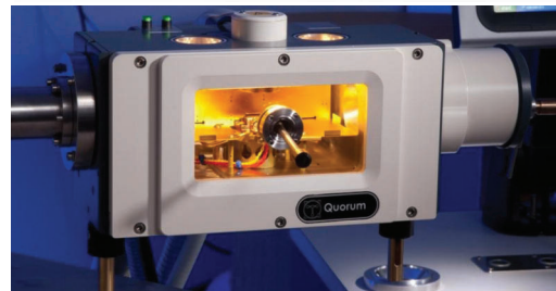
Cryo preparation chamber with cryo transfer device fitted
