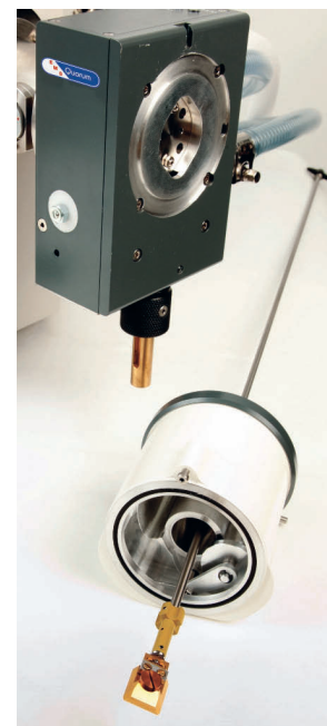
QuickLok and specimen transfer device
