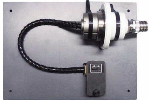
Coolstage and vacuum feed through connected to the storage block (stage protected by plastic shutter)
