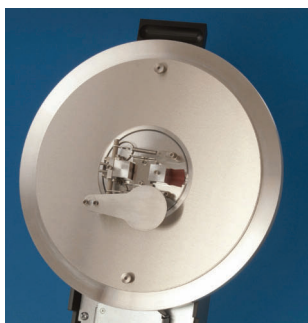
Carbon rod evaporation insert
