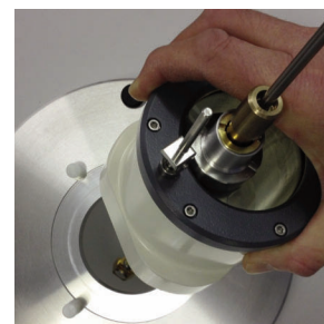
Slushy nitrogen freezing station
