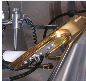
Cold trap - adapted to installation
