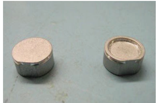
Dish-style specimen stub, showing flat bottom side (left) and dish side (right)
