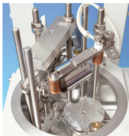
Typical chamber set up, showing carbon and metal evaporation sources, specimen stage and optional film thickness monitor (FTM)
