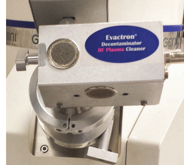
SEM chamber with Evactron® Decontaminator Plasma Radical Source (PRS) attached. An adaptor flange is used to mount the Evactron® Decontaminator to the SEM.
